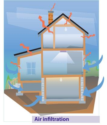
Outside air can enter your house through cracks in your foundation wall, siding, or around windows and doors. Inside (conditioned) air can escape around chimneys, vents, pipes, and wires that penetrate walls, ceilings, and attics.
