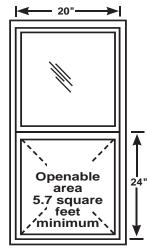
Emergency escape and rescue openings shall be operational from the inside of the room without the use of keys, tools or special knowledge (R319.1.4).
